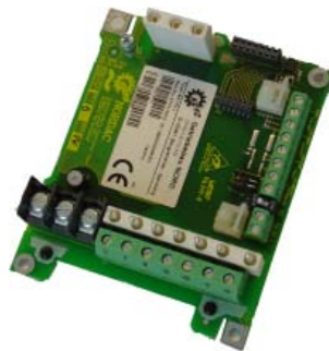
CIU - customer interface unit
