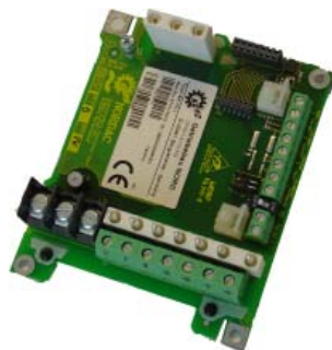
CIU - customer interface unit
