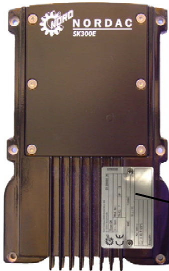
SK 300E with mounted rating plate and without LEDs
