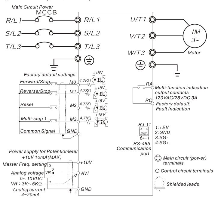
NOTE: Do not plug in a Modem or telephone line to the RS-485 communication port, permanent damage may result. Terminals 1 & 2 are the power source for the optional copy keypad and should not be used while using RS-485 communication.
